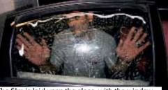
The film is laid upon the glass, with the window slightly down, and the moisture is smoothed out.
