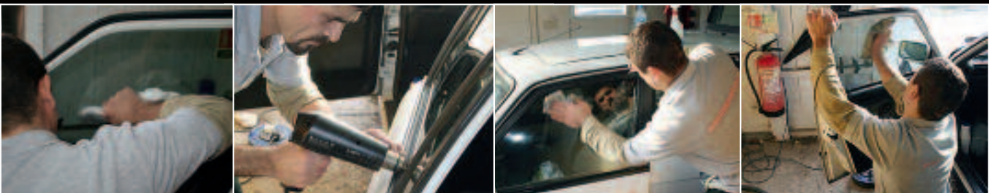
> Cahit uses a squeegee wrapped in a good quality cloth to chase out any remaining air bubbles
